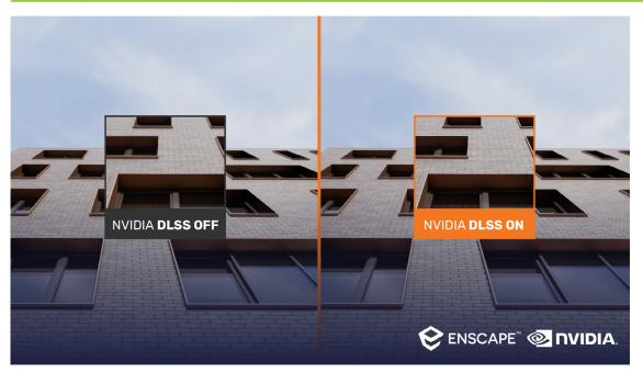
dedicated Tensor Cores in the NVIDIA RTX GPU 'upscale' the image using AI and Machine Learning techniques. To the end user, there is no noticeable loss in image quality, but frame rates can rise dramatically, removing any sign of 'ghosting' as the user navigates around the virtual building.
