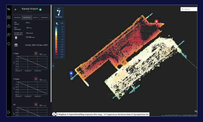
Synspective Land Displacement Monitoring Service originated from InSAR\* analysis that is capable of detecting timely vertical land displacement, in millimeters, over a wide area. This Service enables periodical observation and understanding of land subsidence and deformation.
